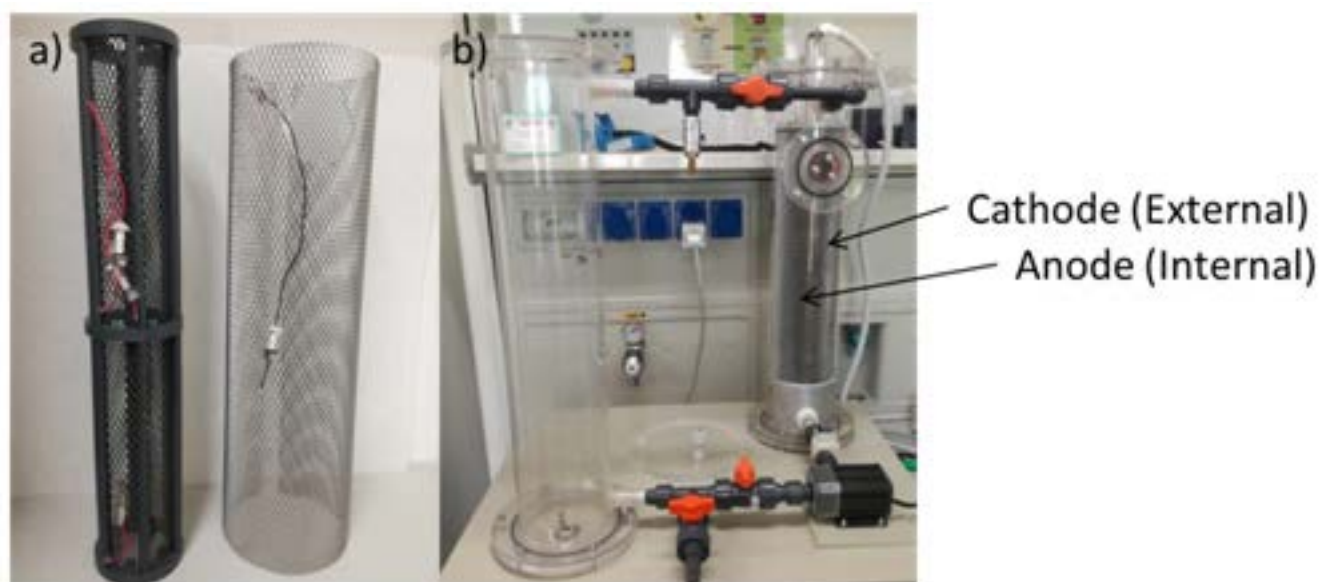
Figure 2. Photograph of a) contacts to anode (left) and to cathode (right); b) insertion of electrochemical apparatus into semi-pilot plant.
