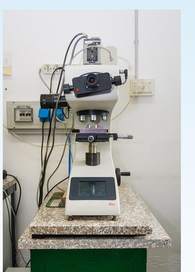
Microindenter Leica VMHT MOT Microhardness of metal-ceramic interfaces
