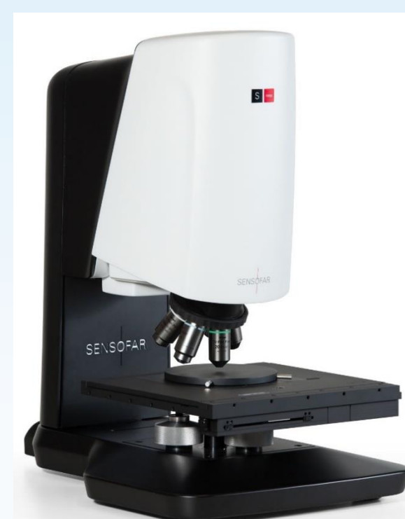
3D Profilometer Sensofar S-Neox confocal+interferometric+focus variation Lateral resolution of the order of nm
