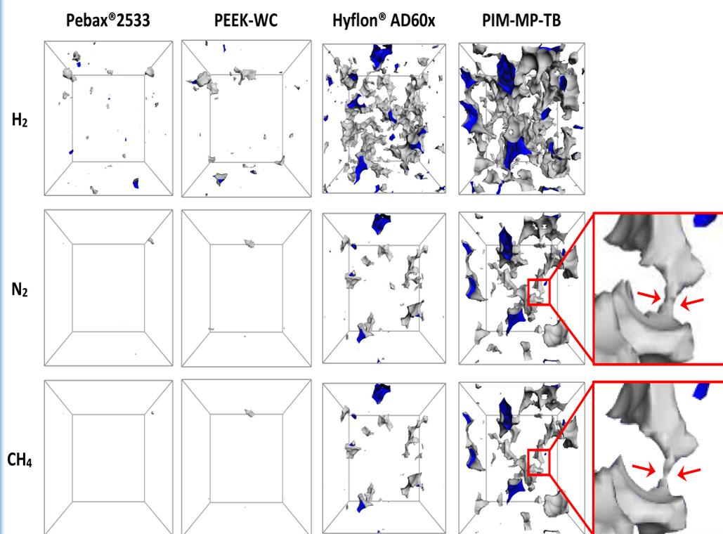
Molecular models showing the accessible fractional free volume for H<sub>2</sub>, N<sub>2</sub> and CH<sub>4</sub> in four polymers. The inserts are zoom-ins of the connection between two free volume elements for N<sub>2</sub> and CH<sub>4</sub>. Grey shading indicates the free volume elements seen from the outside, facing the polymer; blue shading indicates the inside of the free volume elements.
