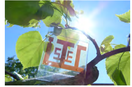
Prototype of Dye Sensitized Solar Cells (DSSC) for building integrated photovoltaics.
