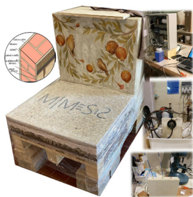
Prototype of historical wall with embedded sensors for pH and chlorides detection.
