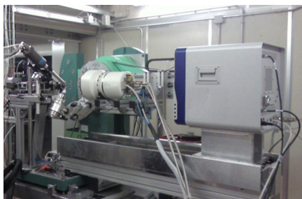
X-Ray Diffraction I (XRD1) beamline at the Elettra synchrotron.
